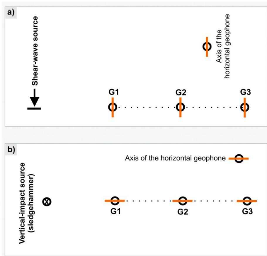
**Figure 2. Data acquisition using only horizontal-component geophones:** a) geophone array for SH-wave refraction and Love-wave dispersion analysis; b) geophone array for Rayleigh-wave analyses (radial component). Please notice that Rayleigh waves can be detected also using vertical-component geophones (which cannot be used for detecting Love waves).
