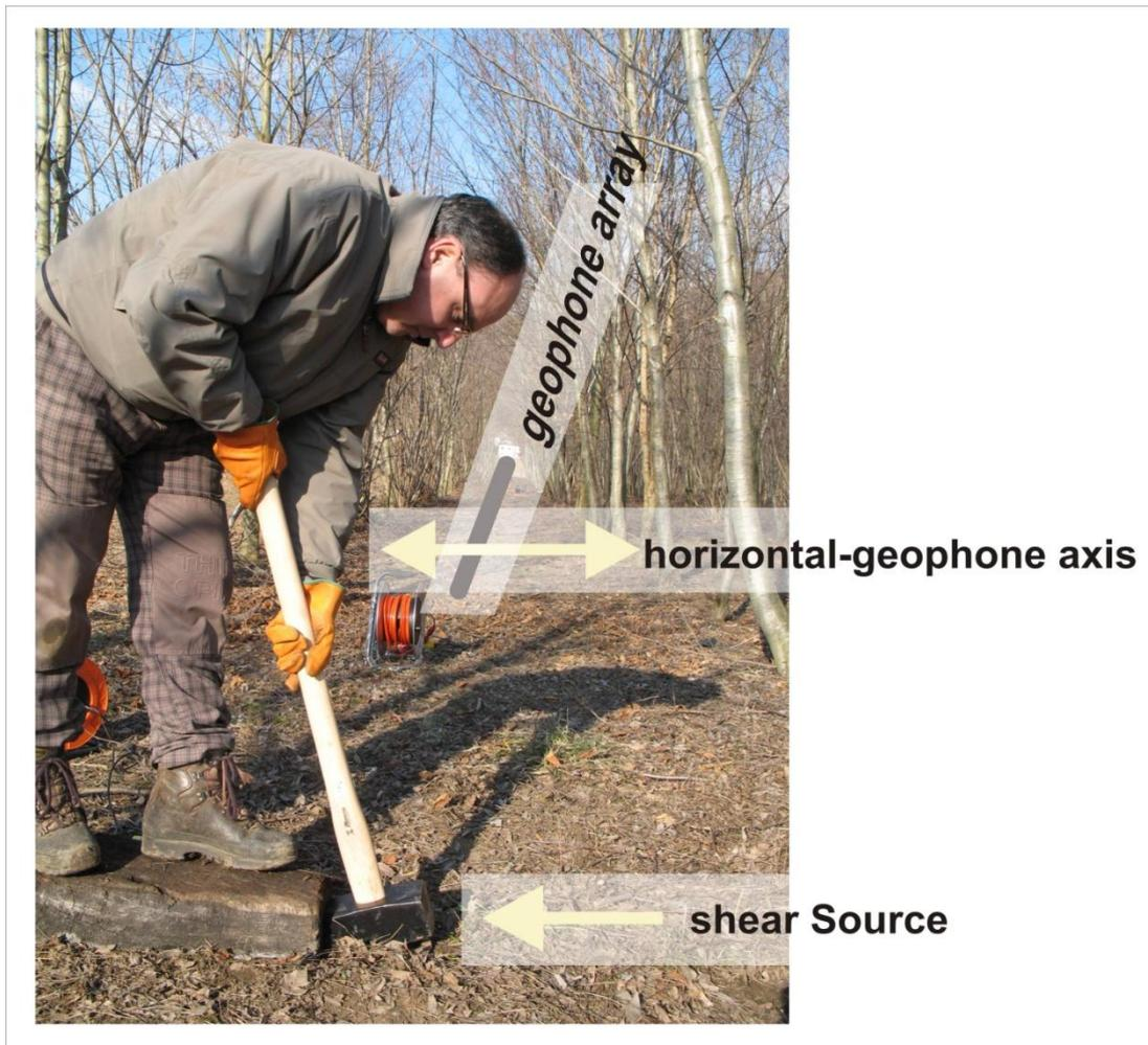
**Figure 3.** Data acquisition for SH-wave refraction travel time determination and Love-wave dispersion analysis (shear source and geophone-axis perpendicular to the array – see Figure 2 as well).
