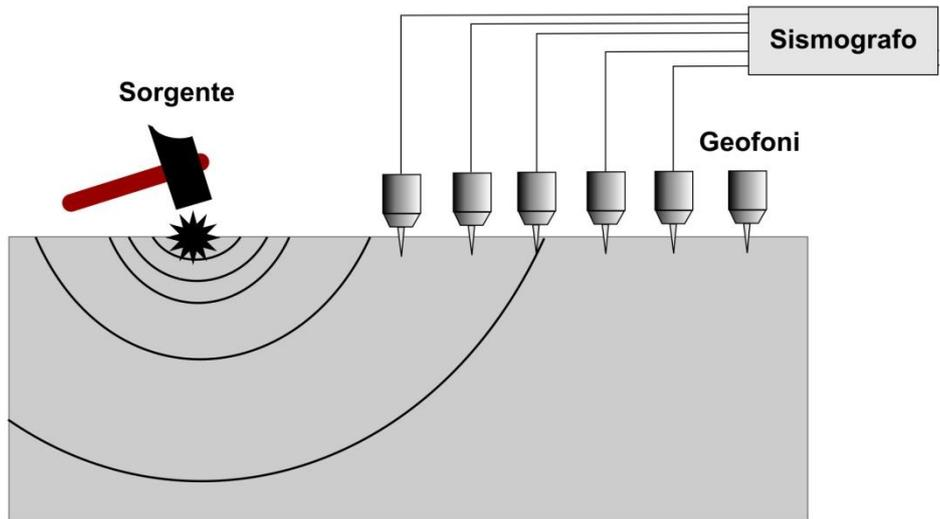
**Figure 1. Seismic source.** In order to acquire data useful for Rayleigh-wave analyses is necessary to deal with vertical-impact source (e.g. the very classical sledgehammer), while for analyzing Love waves (and/or SH-wave refractions) we must generate shear waves through a horizontal-component impact (see also Figures 2 and 3).
