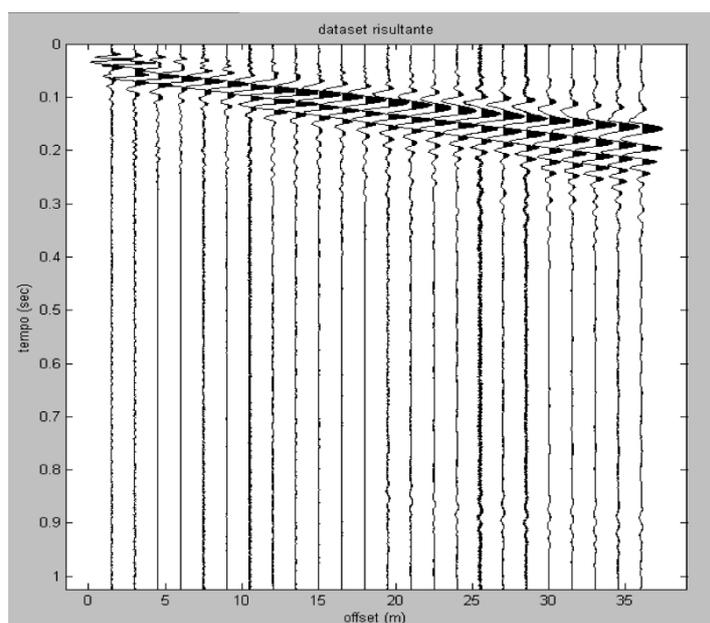
**Figure 5.** Dataset with a correct amplitude (gain values set to proper values).
